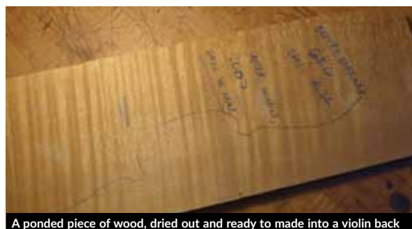
A ponded piece of wood, dried out and ready to be made into a violin back
